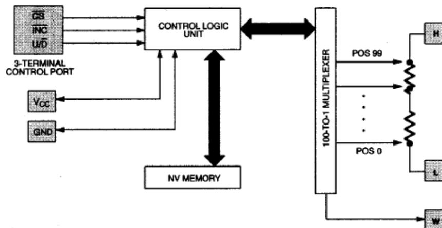
Figure 3. Block Diagram of the Digipot IC
