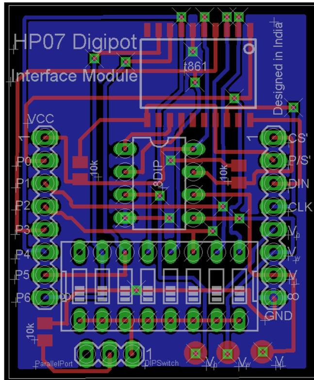
Figure 9. PCB Layout of the module
