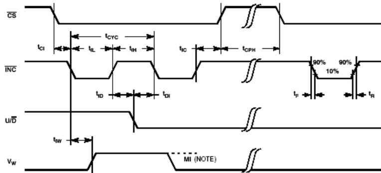
Figure 5. Timing diagram of signals between microcontroller and digipot IC
