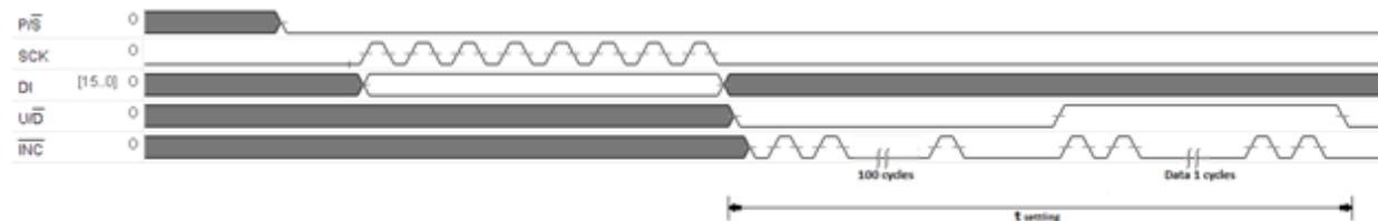
Figure 7. Timing diagram of signals from external source to and from the microcontroller in serial mode
