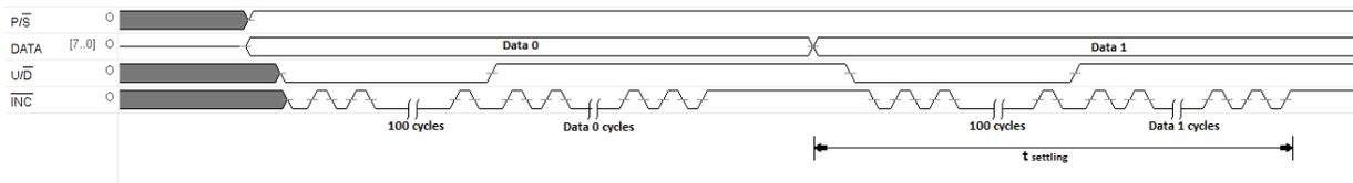
Figure 6. Timing diagram of signals from external source to and from the microcontroller in parallel mode
